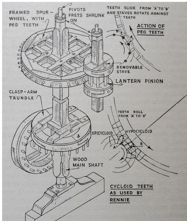
Examples of wooden gearing, and illustration of an improvement made by Rennie
